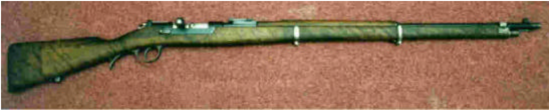
The Model 1886/89, sometimes called the Colonial variant, is the infantry rifle fitted with a clip-on handguard from the front of the sight to the middle barrel band. It is suggested that the handguard was fitted to rifles issued to colonial troops to reduce the effect of difficulty sighting due to radiated barrel heat.
