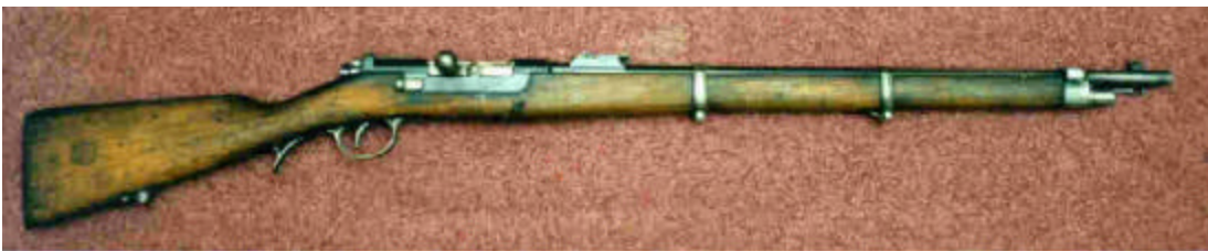
The M1886 Kropatschek Short Rifle. Virtually identical to the infantry rifle except for its length, the sight and a magazine capacity of 6 rounds; (only 4800 were ever produced).
